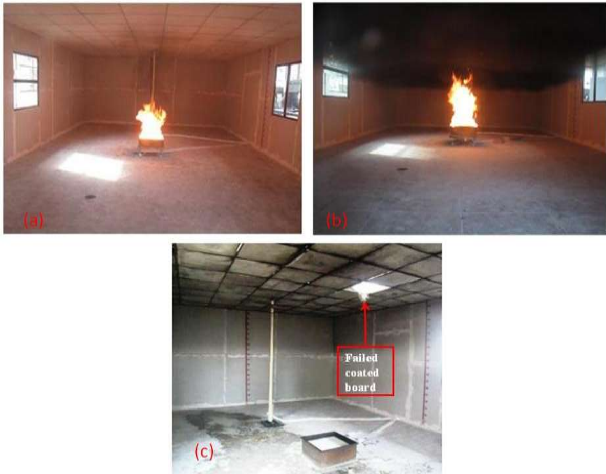
Fig. 5.4 Large room fire study (Expt. #1): (a) beginning (at 4s) of the experiment; (b) at 33 s of the experiment (c) roof condition after 257 s
