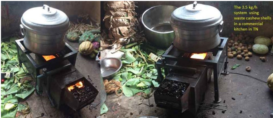
Figure 25: The single pan HC 3 D at about 4 kg/h with a 12 V, 12 W two-stage fan operated with a rechargeable battery burning cashew shell fuel
