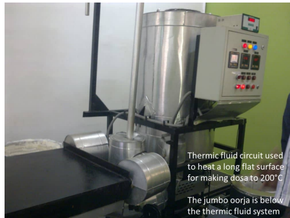
Figure 16: Two 300 mm diameter combustion systems burning built by FEPL for the special application making dosas (thin pan cakes) on large scale using thermic fluid heater that maintains a temperature of 200 \pm 10^\circ on the surface
