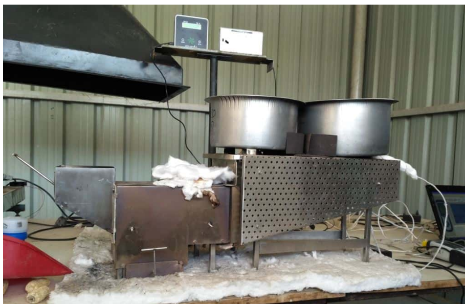
Figure 41: The arrangement for the measurement of emissions. The hood on the left side used for obtaining the stove emissions and on the right meant for obtaining indoor air quality - CO and PM_{2.5}
