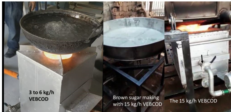
Figure 34: 3 to 6 kg/h for larger cooking and 15 - 20 kg/h VEBCOD operating system for brown sugar production
