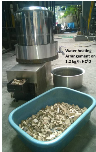
Figure 23: Water heating arrangement mounted on a 1.2 kg/h combustion system to deliver hot water
