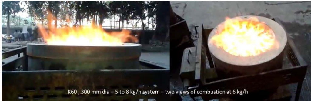
Figure 15: The 300 mm diameter, 5 to 8 kg/h industrial size combustion system burning pellets built by FEPL and marketed in several states in India
