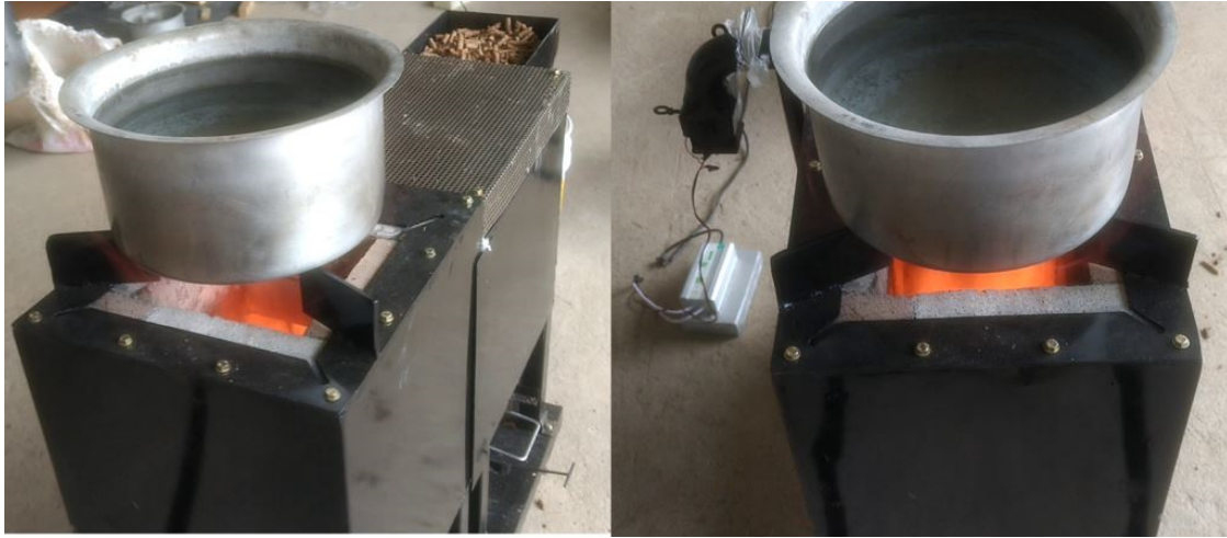
Figure 24: The single pan HC 3 D at 2.5 to 4 kg/h with a 12 V, 12 W two-stage fan operated with a rechargeable battery burning pellet fuel
