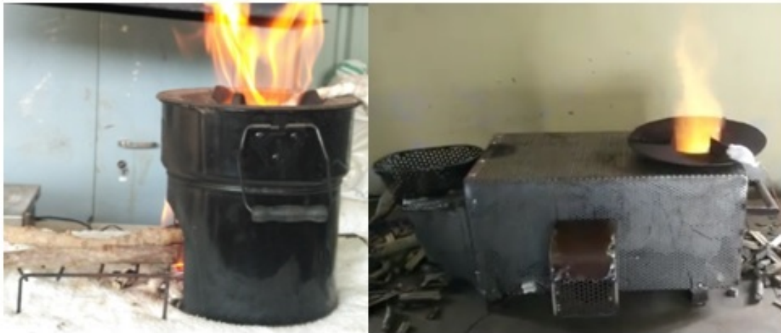
Figure 38: Comparison between the flames behavior of a free convection stove and the single pan forced convection single pan HC 3 D)
