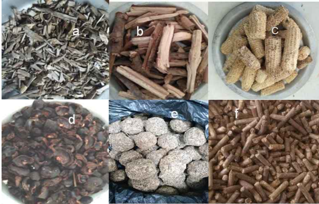
Figure 3: Fuels for small combustion systems: (a) Cut tree droppings along with bark, packing density of 200 to 210 kg/m 3 , (b) caesarina chopped pieces, packing density of 240 to 280 kg/m 3 , (c) corncobs, packing density of 200 to 210 kg/m 3 , (d) cashew shell waste - 90 to 100 kg/m 3 , (e) processed sawdust-cowdung balls, 60 to 80 kg/m 3 , (f) pellets of a mix of seasonal agro-residues, packing density = 600 kg/m 3 , ash content of all biomass \leq 5\% , drawn from Mukunda and Attanoor, 2017
