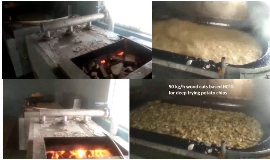
Figure 29: The HC 3 D at about 50 kg/h with wood cuts from a wood processing industry for potato chip deep frying; the off-cuts used in the combustion system are clearly visible
