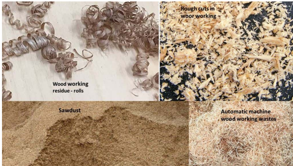
Figure 2: Wood processing based fine biomass, packing densities of 50 to 100 kg/m 3 that need pre-processing for use in combustion systems
