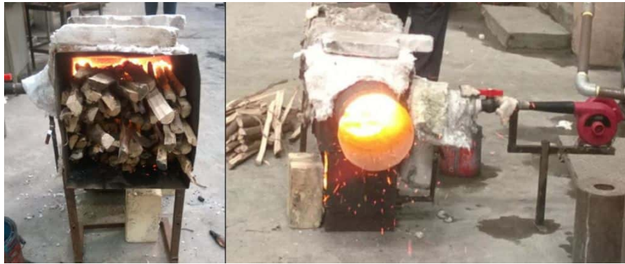
Figure 18: The first experiments with firewood and only a secondary air supply from a high speed blower in the horizontal mode
