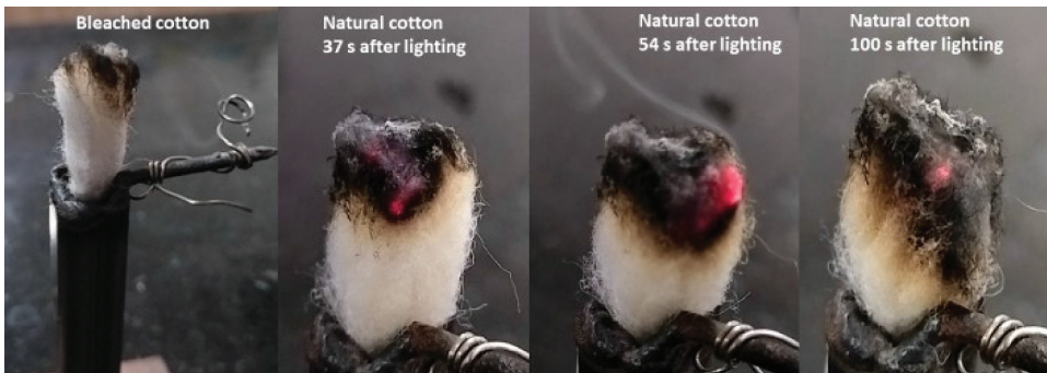
Figure 11. Pictures of smouldering of cotton strand, d = 25 \text{ mm} , \rho_f = 70 \text{ kg/m}^3 at different times.
