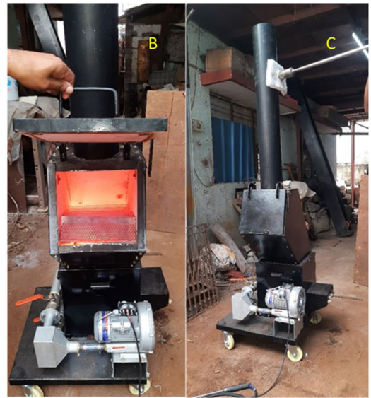
Figure 14: The 3.5–6 kg/h VEBCOD system arranged for the combustion of sanitary pads and diapers. Inset A shows the schematic of the system and B shows the system in combustion mode and inset C , the set up for emission measurements.
