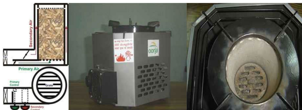
Figure 4: The reverse downdraft stove: fixed volume loaded pellet fuel (largely), gasification air supply from the bottom, combustion air from the top holes both needing a fan of 1.5 We for 3 kWth power from the combustion system.
