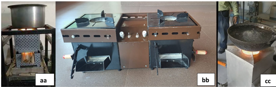
Figure 13: VEBCOD—Examples of single pan 1 kg/h system (aa), two pan version of 1 kg/h each (bb) and 3.5 to 6 kg/h (cc) largely for use with long sticks—split coconut or palm frond, firewood, corncob, etc.
