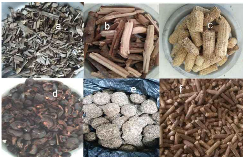
Figure 10: Fuels for small combustion systems: a cut tree droppings along with bark, packing density of 200–210 kg/m 3 . b Causarina chopped pieces, packing density of 240–280 kg/m 3 , c corncobs, packing density of 200–210 kg/m 3 , d cashew shell waste—90–100 kg/m 3 , e processed sawdust-cowdung balls, 60–80 kg/m 3 , f pellets of a mix of seasonal agro-residues, packing density = 600 kg/m 3 ; ash content < 5%, drawn from 11 .
