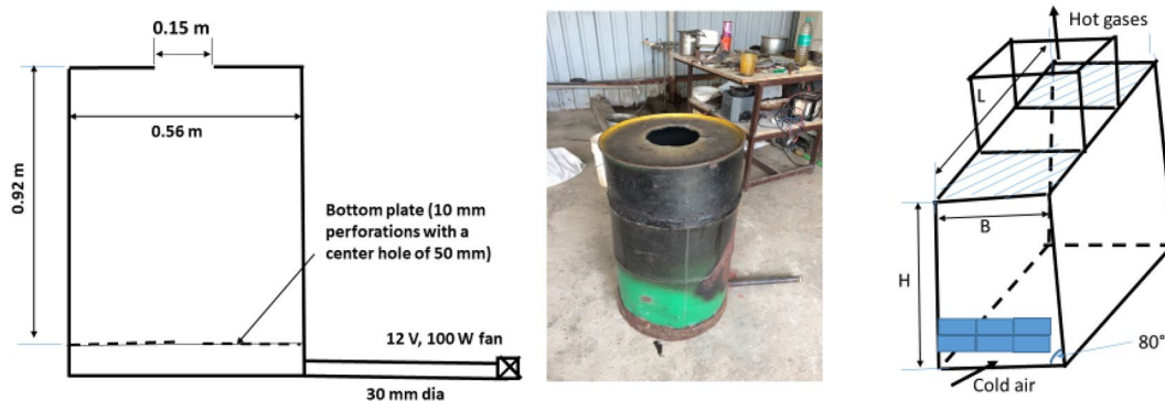
Figure 6: The simple biochar production systems—a 0.56 m diameter, 200 L waste diesel drum based reactor on the left for many light residues and the brickwork based reactor on the right for bales of rice straw.
