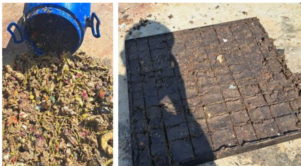
Figure 11: The in-feed waste material received from M/s carbon masters and the processed cakes that can be used as combustible material in domestic or industrial combustion systems.
