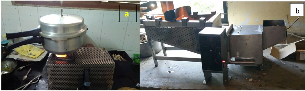
Figure 12: HC 3 D—single pan (a) and two pan (b) versions with chipped wood. Many other fuels in Fig. 10 acceptable for operation.
